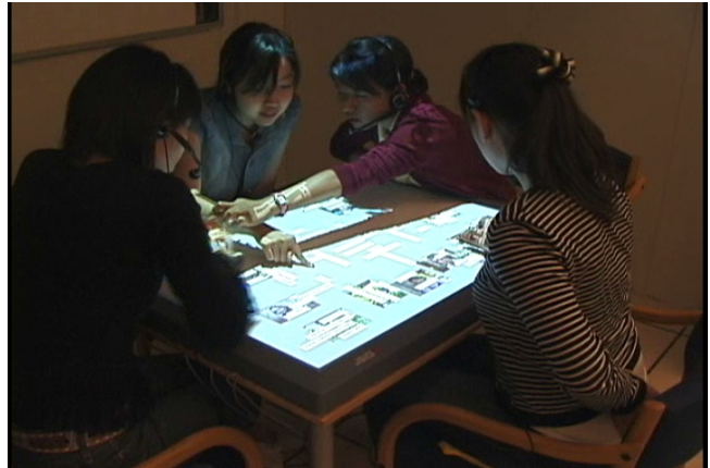
Figure 1. Four students sit around a touch-sensitive DiamondTouch table, working together to match pictures with words in a foreign language, using the MatchingTable software.
